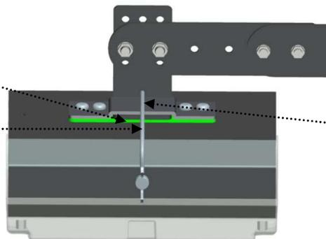
3. If the metal cord is not tight, adjust the length, and **MAKE SURE THE CORD IS TIGHT!**
